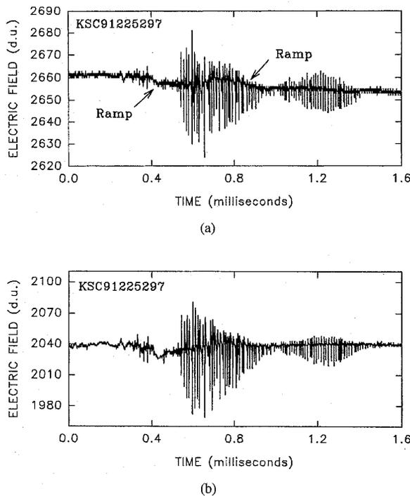
Fig. 6. A sequence of two regular pulse bursts associated with small ramplike field changes (*K*-changes) in a cloud discharge; (a) Decay time constant of 10 s ("slow antenna" trace); (b) Decay time constant of 150  $\mu$ s ("fast antenna" trace). Note that the gain for Fig. 6(a) is about an order of magnitude higher than for Fig. 5(a), while the gain for Figs. 6(b) and 5(b) is the same. Positive field change deflects downward (atmospheric electricity sign convention).
