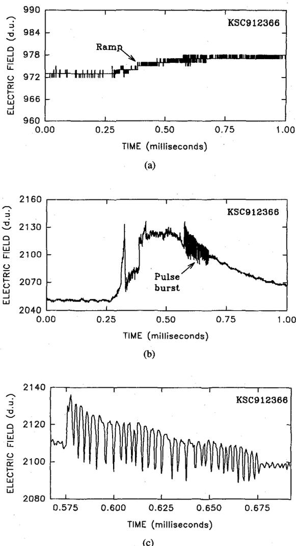
Fig. 5. A regular burst of microsecond-scale pulses associated with a ramp-like millisecond-scale field change (*K*-change) in a cloud flash; (a) Low gain, decay time constant of 10 s ("slow antenna" trace); (b) High gain, decay time constant of 150  $\mu$ s ("fast antenna" trace); (c) Portion of (b) showing the regular pulse burst on an expanded time scale (25  $\mu$ s per division). Positive field change deflects downward (atmospheric electricity sign convention).
