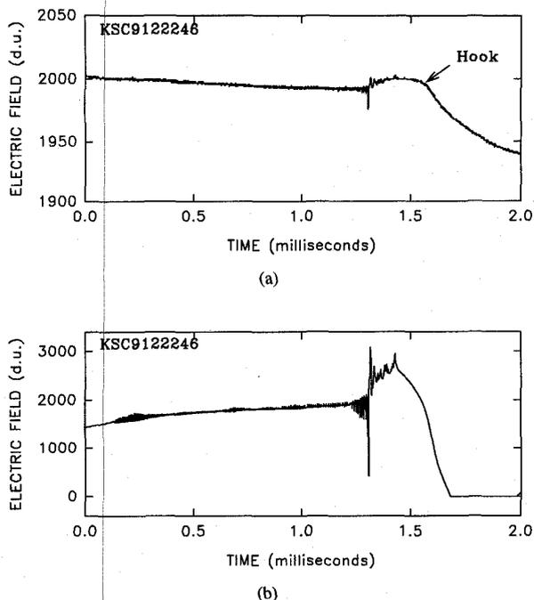
Fig. 3. Regular bursts of microsecond-scale pulses associated with a hook-shaped millisecond-scale field change (*M*-change); (a) Low gain, decay time constant of 10 s ("slow antenna" trace); (b) High gain, decay time constant of 150  $\mu$ s ("fast antenna" trace). The pulses are shown on an expanded time scale in Fig. 4.
