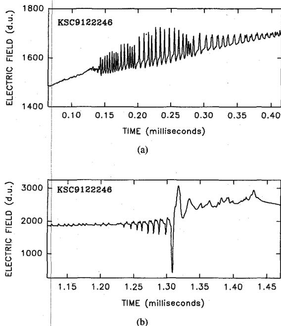
Fig. 4. Two fragments of the field record shown in Fig. 3(b) but on an expanded time scale (50  $\mu$ s per division). Positive field change deflects downward (atmospheric electricity sign convention).
