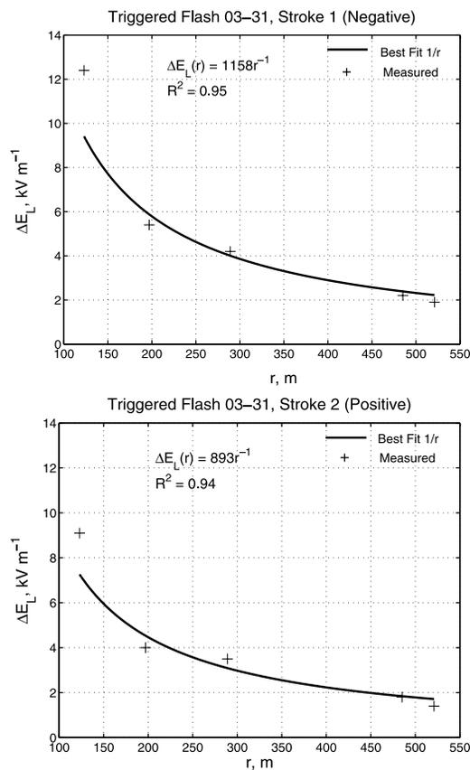
**Figure 6.** Plots of the first (top) and second (bottom) stroke leader electric-field change versus distance as measured from waveforms recorded at five stations located 120 to 520 m from the lightning channel. The best-fit inverse distance dependence curve (solid line) is plotted along with the measured data. The waveforms recorded at 120 m are shown in Figure 3.
