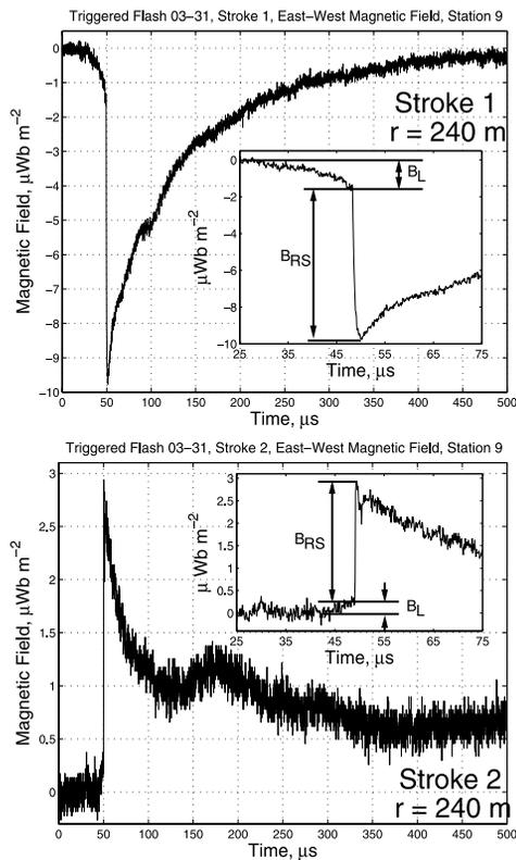
**Figure 4.** First (negative, top) and second (positive, bottom) stroke magnetic field waveforms, measured 240 m from the channel. Only the east-west component was measured, with the angle between the plane of the loop antenna and the direction of the launcher being approximately 20 degrees. The insets show the waveforms expanded on 50  $\mu\text{s}$  time scales. The leader ( $B_L$ ) and return stroke ( $B_{RS}$ ) portions of the waveforms are labeled.
