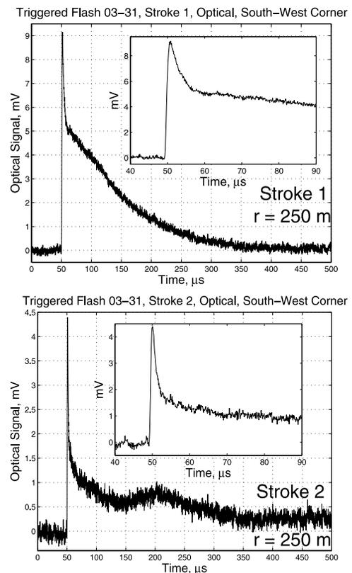
**Figure 5.** First (top) and second (bottom) stroke luminosity waveforms, measured at the south-west corner of the network, approximately 250 m from the channel. The insets show the waveforms expanded on 50  $\mu\text{s}$  time scales.
