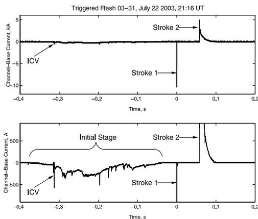
**Figure 1.** Overall flash current records. The initial stage, the initial current variation (ICV), and the two return strokes are labeled. The top and bottom records are displayed on the same time scale but on high and low amplitude scales, respectively. The bottom record is clipped (both polarities) at 900 A.
