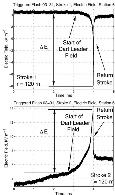
**Figure 3.** First (top) and second (bottom) stroke electric field waveforms, measured approximately 120 m from the channel. The start of the leader field and return stroke portion of the waveforms are labeled.
