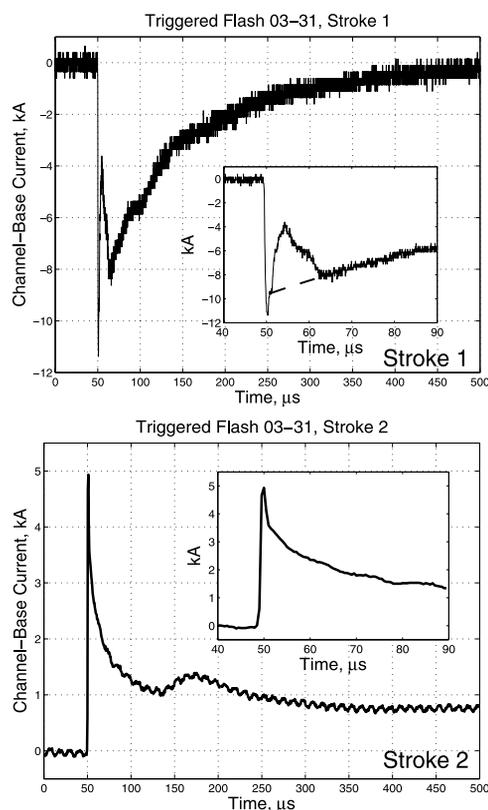
**Figure 2.** First (negative, top) and second (positive, bottom) return stroke current waveforms. The first stroke waveform was obtained from the high-bandwidth (5 MHz) record while the second stroke waveform was obtained from the low-bandwidth (500 kHz) record. The insets show the waveforms expanded on 50  $\mu$ s time scales. The dotted line shown in the top inset is a hypothetical reconstruction of the current lost due to the flashover.
