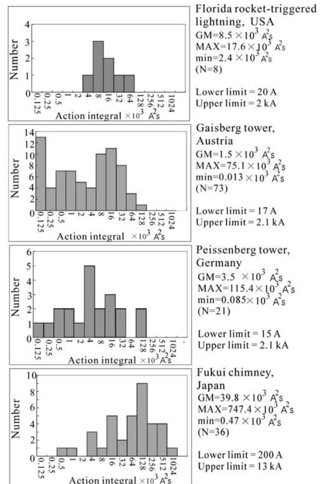
**Figure 10.** Histograms of the action integral ( $\int i^2 dt$ ) of the initial stage. The geometric mean (GM), maximum (MAX), and minimum (min) values are indicated beside each histogram. Sample sizes are given in parentheses. The action integral was evaluated from the low-level current record. The lower (upper) current measurement limit was 200 A (13 kA) for the Fukui data set and 15–20 A (2–2.1 kA) for the other three data sets.
