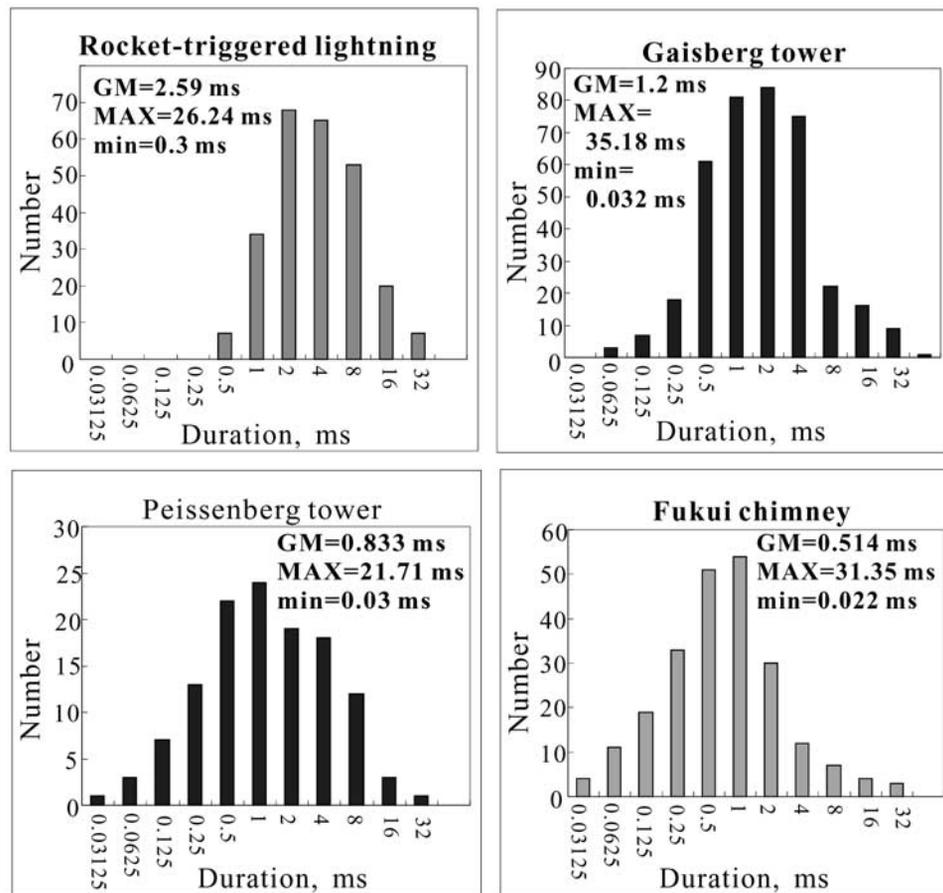
**Figure 12.** Histograms of the duration of ICC pulses. The geometric mean (GM), maximum (MAX), and minimum (min) values are indicated on each histogram.
