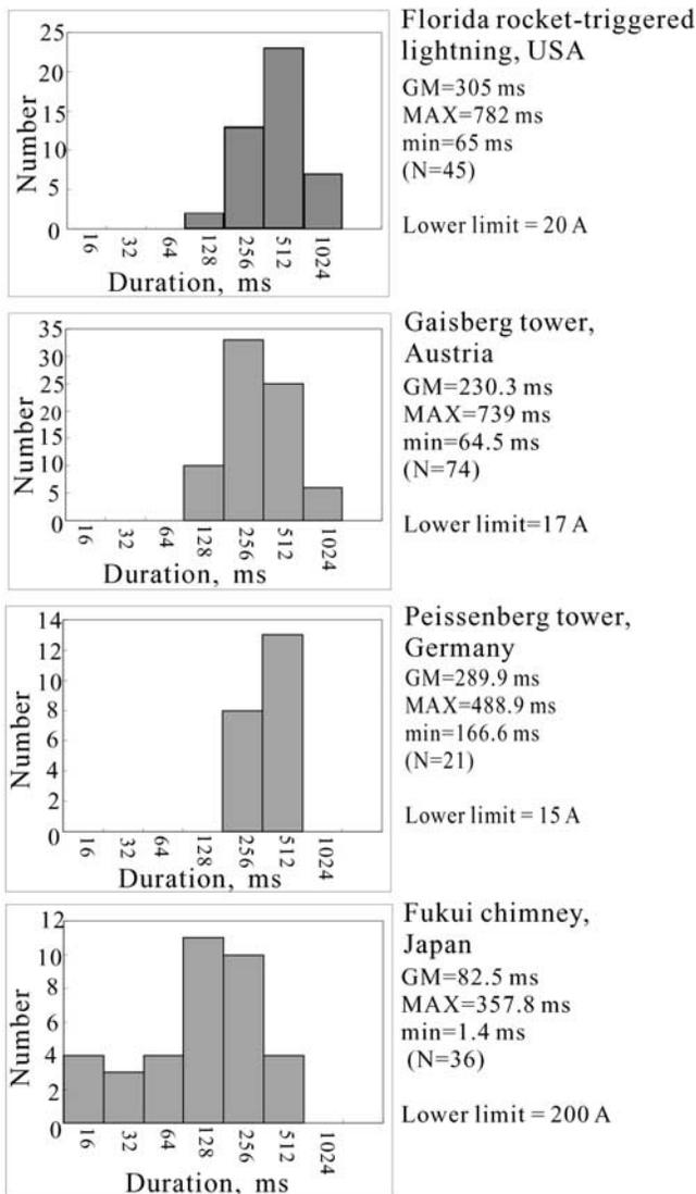
**Figure 7.** Histograms of the duration of the initial stage. The geometric mean (GM), maximum (MAX), and minimum (min) values are indicated beside each histogram. Sample sizes are given in parentheses. The lower (upper) current measurement limit was 200 A (13 kA) for the Fukui data set and 15–20 A (2–2.1 kA) for the other three data sets.
