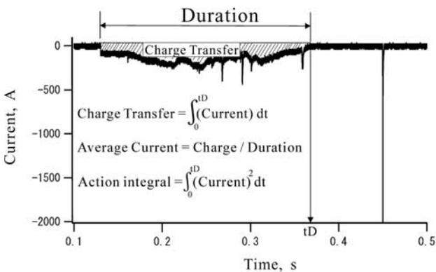
**Figure 5.** Definitions of overall characteristics (duration, charge transfer, average current, and action integral) of the initial stage in upward flashes, illustrated using the current waveform shown in Figure 1.
