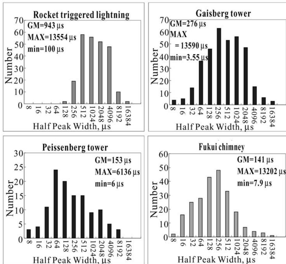
**Figure 14.** Histograms of the half-peak width of ICC pulses. The geometric mean (GM), maximum (MAX), and minimum (min) values are indicated on each histogram.
