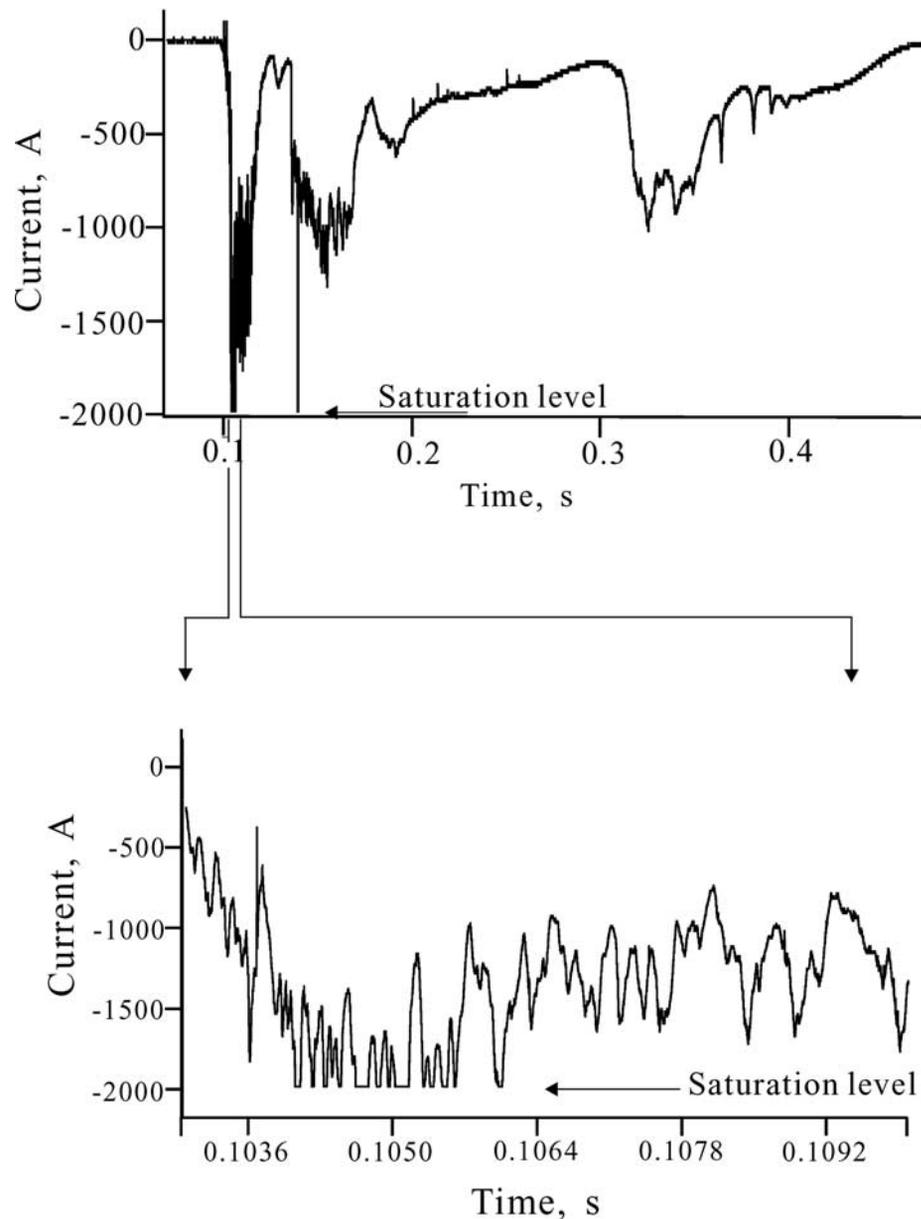
**Figure 17.** Current waveforms of the initial stage exhibiting pulsations during its initial portion in a Peissenberg tower flash (see section 4.2).
