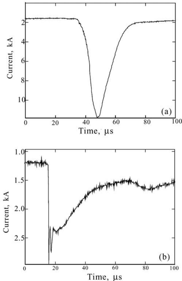
**Figure 15.** Examples of waveshapes of ICC pulses. (a) Slow rise pulse (risetime 7.9  $\mu\text{s}$ ); (b) fast rise pulse (risetime 0.4  $\mu\text{s}$ ).
