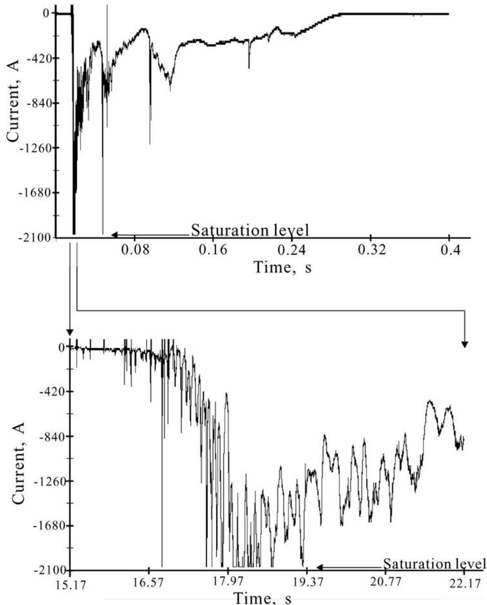
**Figure 16.** Current waveforms of the initial stage exhibiting pulsations during its initial portion in a Gaisberg tower flash (see section 4.2).
