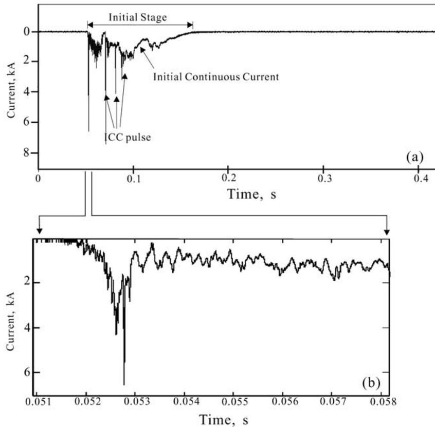
**Figure 4.** (a) Overall current waveform of the initial stage not followed by return stroke pulses in an upward flash at the Fukui chimney, Japan; (b) initial portion of the IS that shows pulsations (see section 4.2).
