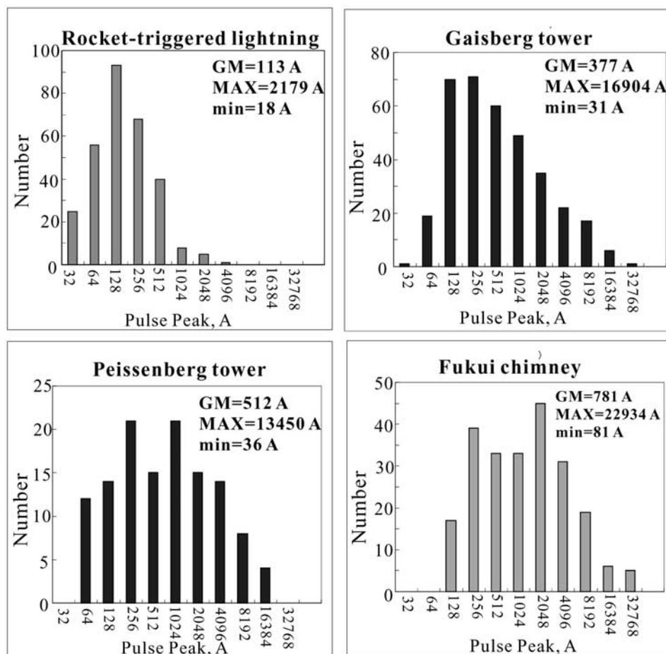
**Figure 11.** Histograms of the peak of ICC pulses. The geometric mean (GM), maximum (MAX), and minimum (min) values are indicated on each histogram.
