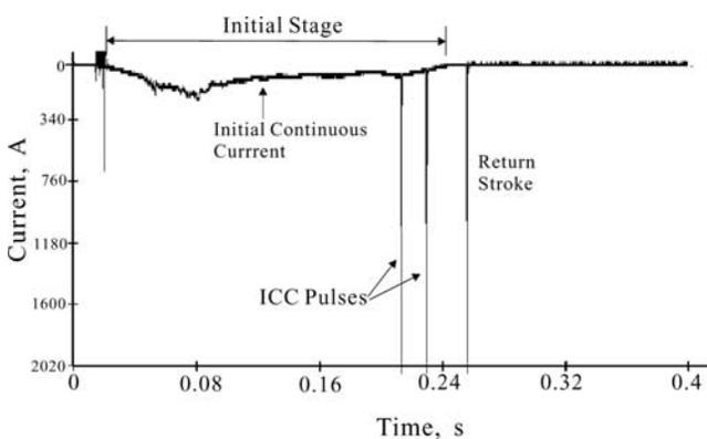
**Figure 2.** Overall current waveform of the initial stage followed by one return stroke pulse in an upward flash at the Gaisberg tower, Austria.
