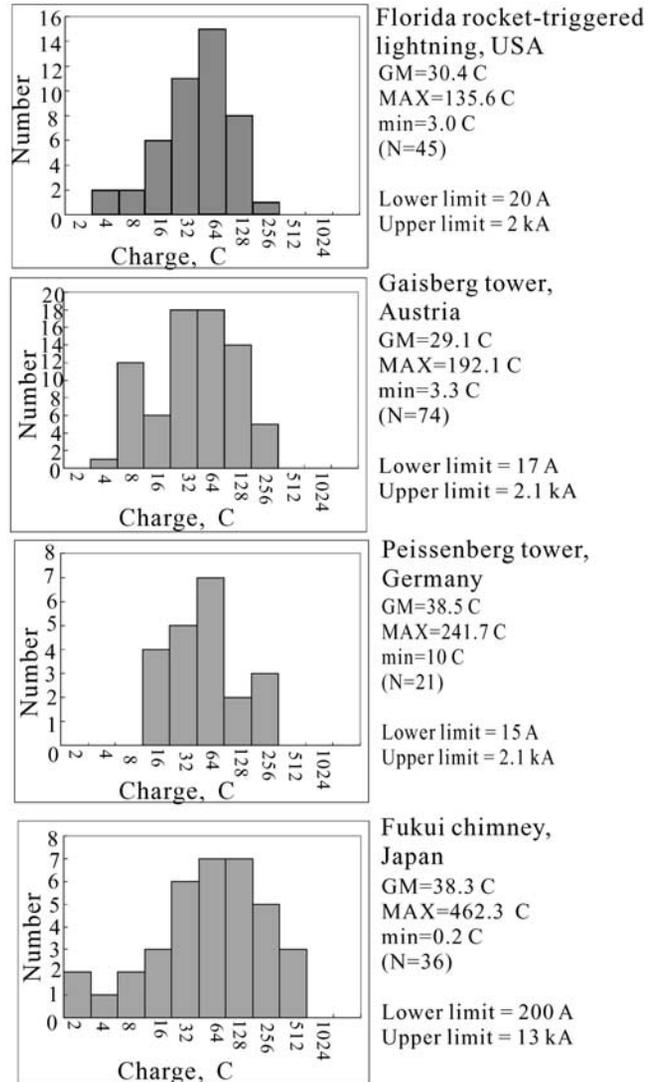
**Figure 8.** Histograms of the charge transfer of the initial stage. The geometric mean (GM), maximum (MAX), and minimum (min) values are indicated beside each histogram. Sample sizes are given in parentheses. The charge transfer was evaluated from the low-level current record. The lower (upper) current measurement limit was 200 A (13 kA) for the Fukui data set and 15–20 A (2–2.1 kA) for the other three data sets.
