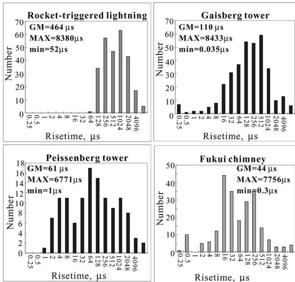
**Figure 13.** Histograms of the risetime of ICC pulses. The geometric mean (GM), maximum (MAX), and minimum (min) values are indicated on each histogram.
