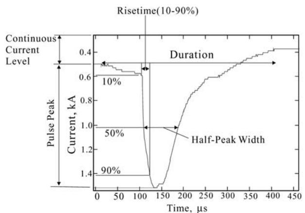
**Figure 6.** Definitions of the parameters (peak, duration, risetime, and half-peak width) of ICC pulses.
