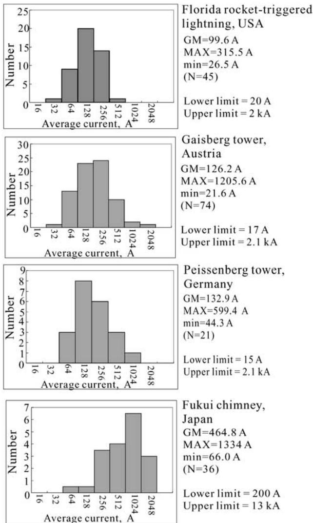
**Figure 9.** Histograms of the average current of the initial stage. The geometric mean (GM), maximum (MAX), and minimum (min) values are indicated beside each histogram. Sample sizes are given in parentheses. The lower (upper) current measurement limit was 200 A (13 kA) for the Fukui data set and 15–20 A (2–2.1 kA) for the other three data sets.
