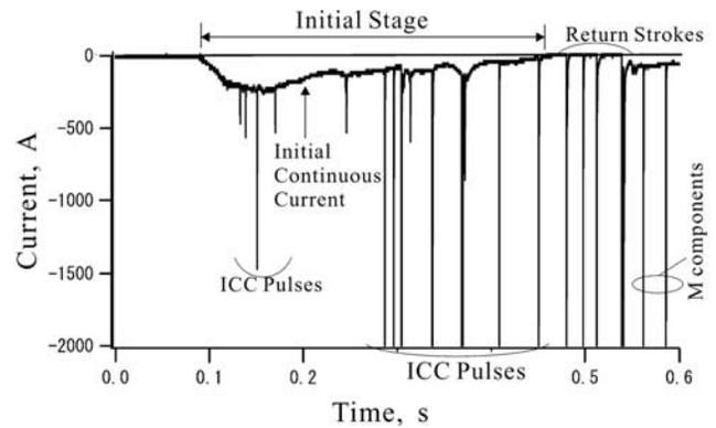
**Figure 3.** Overall current waveform of the initial stage followed by four return stroke pulses in an upward flash at the Peissenberg tower, Germany.
