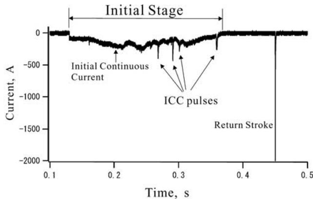
**Figure 1.** Overall current waveform of the initial stage followed by one return stroke pulse in Florida rocket-triggered lightning.
