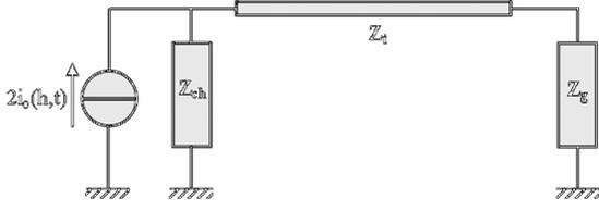
**Figure 3.** Equivalent circuit for the tower struck by lightning (Equation (19)).  $i_o$  is the ‘undisturbed current’.  $Z_{ch}$  and  $Z_t$  are the characteristic impedances of the lightning channel and of the tall strike object respectively.  $Z_g$  is the equivalent grounding impedance.
