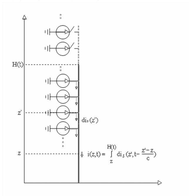
**Figure 1.** Distributed-source representation of the lightning channel in engineering return-stroke models for the case of no strike object and no reflections at ground.
